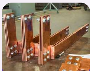
Copper Bus Bars
