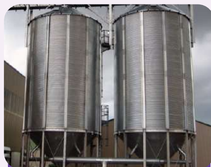
Hopper Silos/ Hopper tanks
